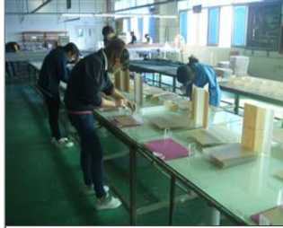
Photo of non-conformity NC Not wearing with rubber gloves in gluing workshop.JPG
