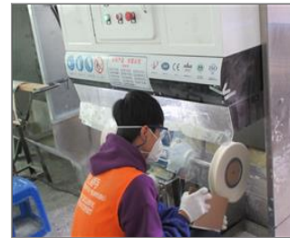
Photo of the personal protection equipments (if applicable) Polishing worker with PPE as mask goggles gloves.JPG
